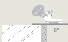
0° router table for untreated surfaces
